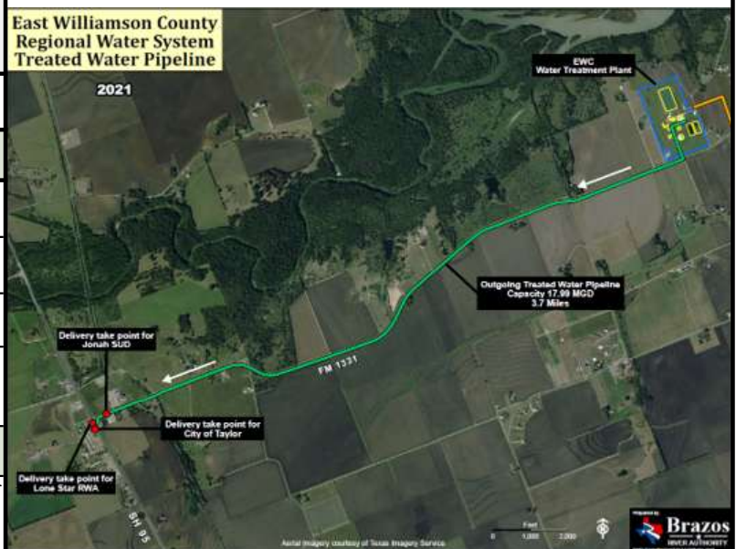
Pictured above: Proposed Treated Water Pipeline alignment
